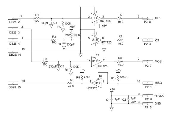
Figure 2.5.3: Logic Level Shifting and Conditioning Circuit
